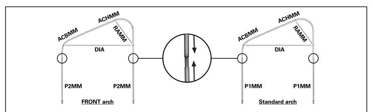
**4.** Add the 2 holes leg (**P2MM**) to both sides of the arch corners for the FRONT arch.
