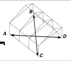
**13**. Install the shelter cover (**T**) on the structure. Tightly attach the tarp with the ties and the rope.
